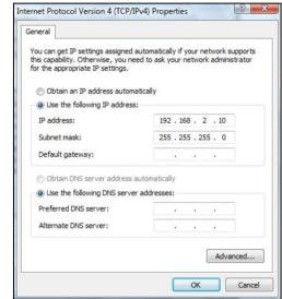
If you changed the AP Controller's IP address, or if your gateway/router uses a DHCP server, ensure you enter the correct IP address. Refer to your gateway/router's settings.
