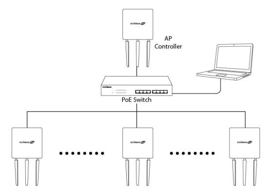
**5.** Open a web browser and enter the AP Controller's IP address in the address field. The default IP address is **192.168.2.2**
