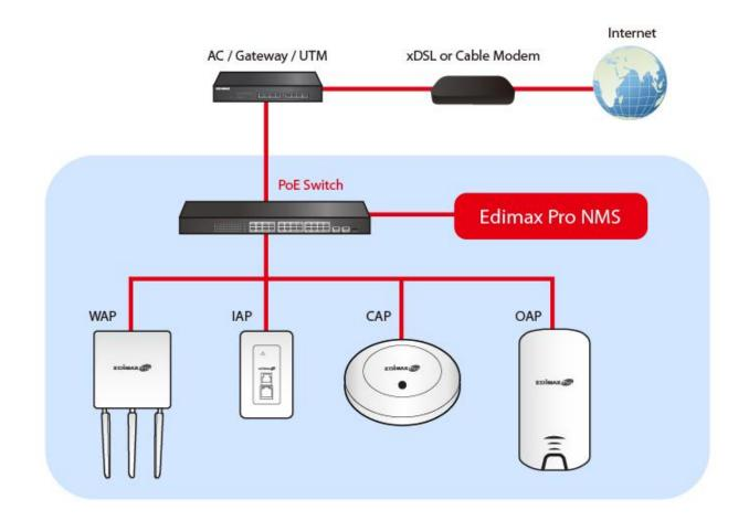
One AP (access point) is designated as the AP Controller (master) and other connected Edimax Pro APs are automatically designated as Managed APs (slaves). Using Edimax Pro NMS you can monitor, configure and manage all Managed APs (up to 16) from the single AP Controller.
